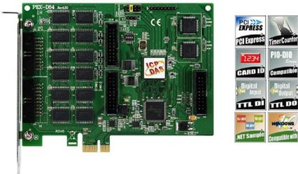
The PEX-D64 card is a new generation product provided by ICP DAS to meet RoHS compliance requirement and is completely compatible with the PIO-D64 series. Users can replace the PIO-D64 series by the PEX-D64 directly without software/driver modification. The PEX-D64 card supports PCI Express bus. It provides 32-ch digital input and 32-ch digital output that consist of two 16-bit input ports and two 16-bit output ports.....[more](#)
