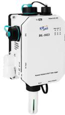
The DL-1000 is a series of particle and gas measurement module that can measure the concentration of aerosols such as PM1, PM2.5, PM10 and the number of particles (0.3 $\mu$ m, 0.5 $\mu$ m, 1 $\mu$ m, 2.5 $\mu$ m, 5 $\mu$ m, 10 $\mu$ m) in the air. In addition, a variety of fume concentrations such as CO/CO2 which may be harmful to human health can also be measured. DL-1000 can trigger an alarm when the concentration is too high.....[more](#)
