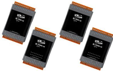
The M-7058-16/M-7059-16 module offers 16 channels for AC/DC digital input, each of which features channel to channel photocouple isolation, and two channels for digital output. All digital input channels are also able to be used as 16-bit counters. The M-7058D-16/M-7059D-16 module has 16 LED indicators that can be used to monitor the status of the digital input channels.....[more](#)
